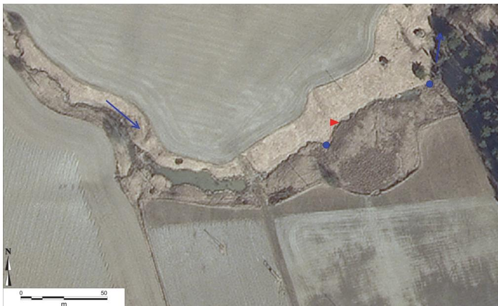
Figure 9. Location of the ferric sulphate doser (marked with red flag) and water quality monitoring spots (marked with blue points).<sup>1</sup>
