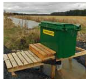
The iron sulphate box is the source of the chemical-containing sock.
